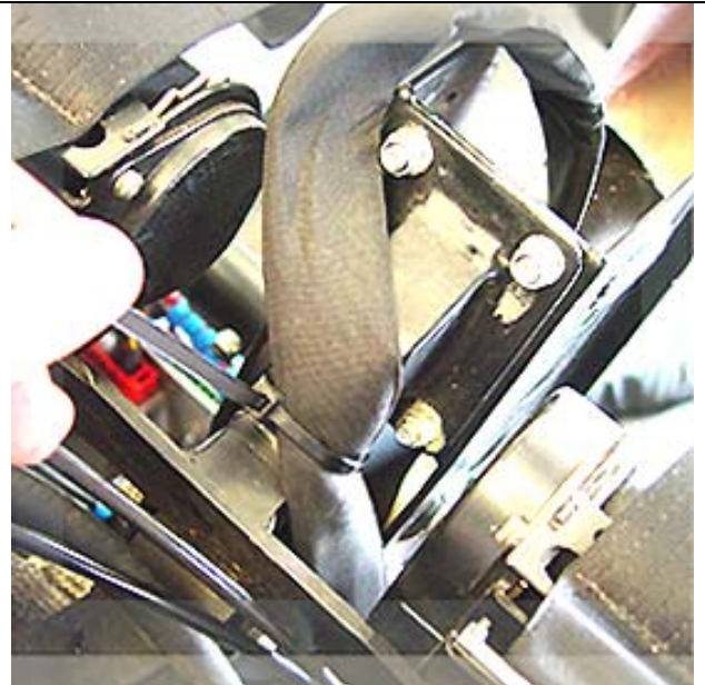
Figure 2-15: The L-shaped, welded, square rod, and the 84" Safety Harness following the cable-tie.
