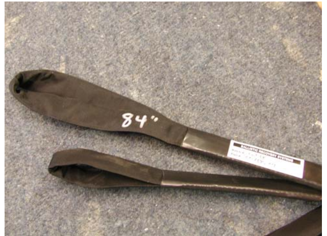
Figure 2-2: The 84-inch Safety Harness
