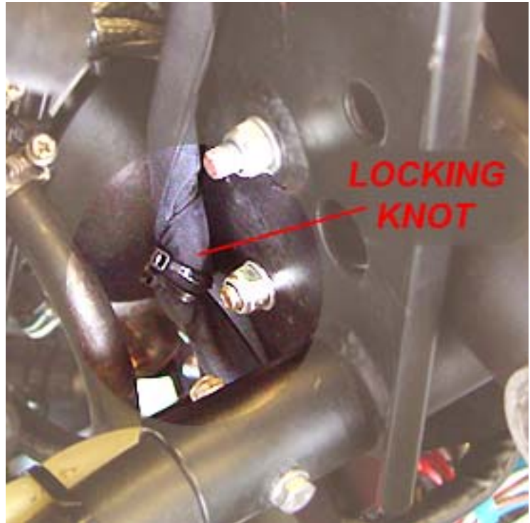
Figure 2-17: Two cable-ties securing the 84" Safety Harness locking knot.
