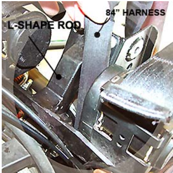
Figure 2-14: The L-shaped, welded, square rod, and the 84" Safety Harness.
