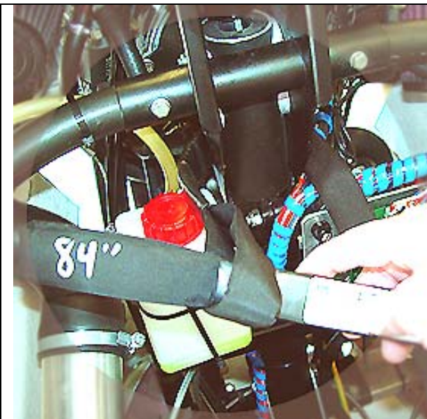
Figure 2-6: The free end of the harness pictured after passing through the open loop.
