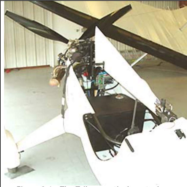
Figure 2-1: The Trike's vertical mast, shown lowered.
