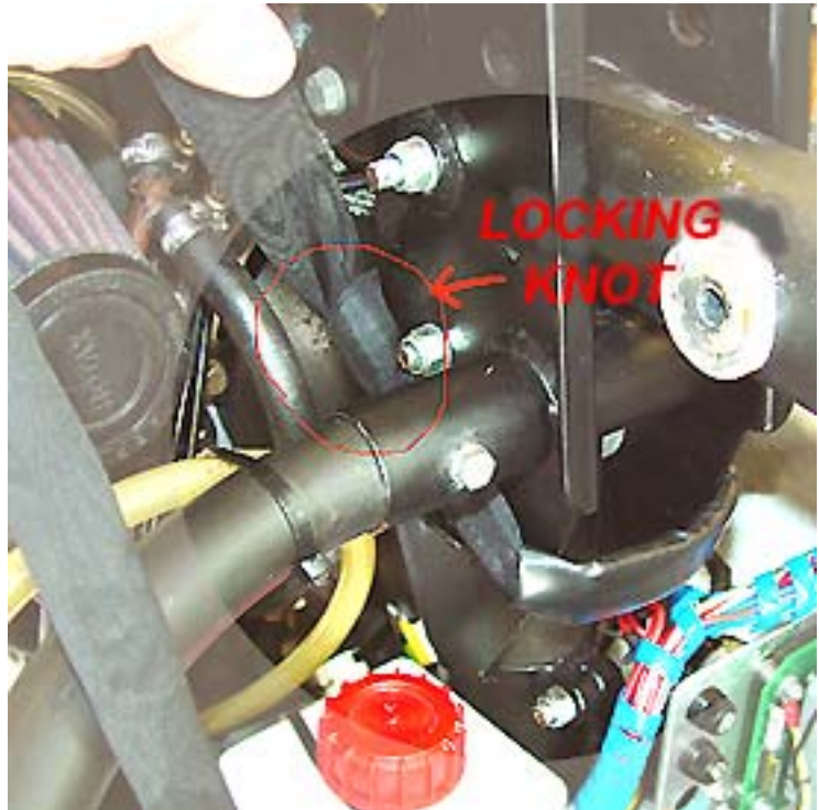
Figure 2-12: The main bracket, with a red circle around the Harness locking knot.
