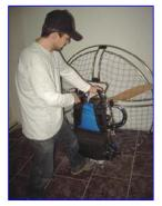
Your left arm holding the throttle should be positioned across the top of the harness or on the SPD whilst you grab hold of the pull start handle with your right hand. Do not leave the
