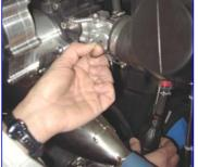
Take the priming pump in on hand and give it one or two good squeezes. Then with your other hand, gently press the carburettor's diaphragm decompressor using the tip of the black cable tie provided.
